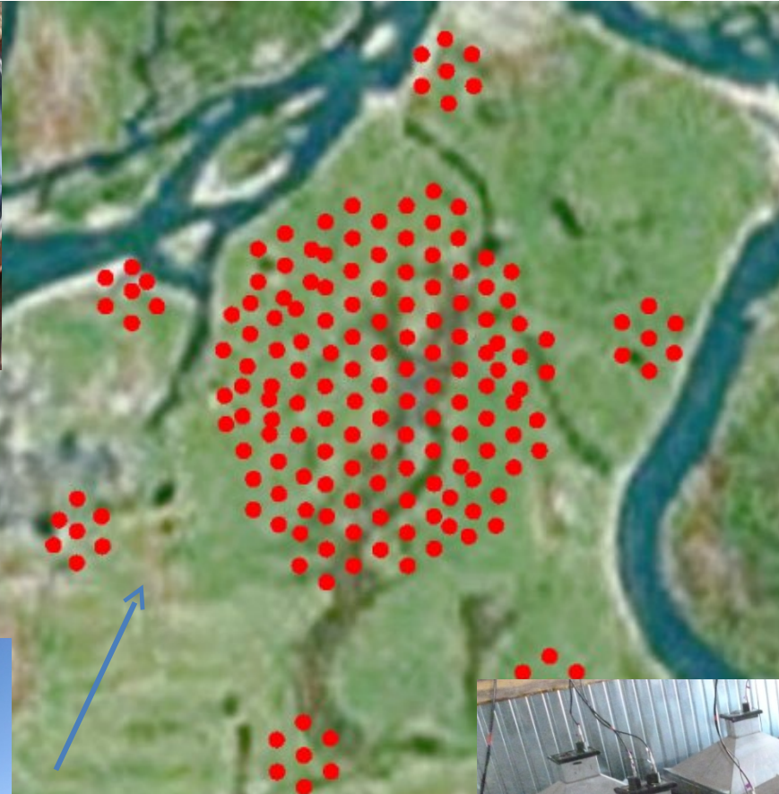
Tunka-Grande – 380 scintillation counters for registration of charged particles
