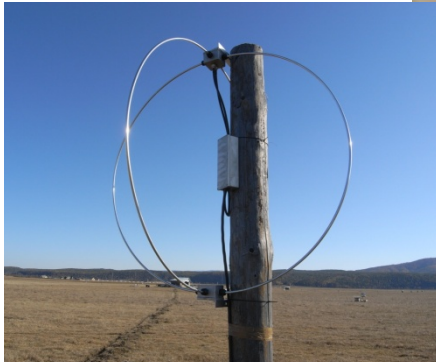
Тунка-REX – 63 antennas for registrations of radio signals From EAS
