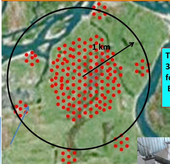
**Tunka- Grande – 380 scintillation counters for detection of EAS charged particles**
